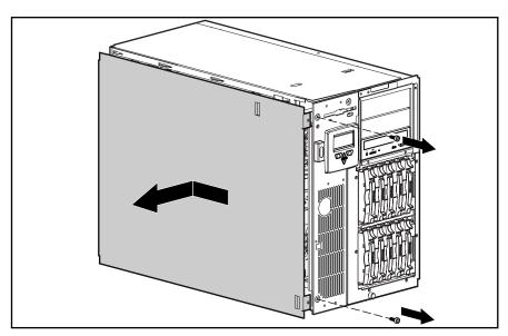
Figure 2-8. Removing the side access panel
